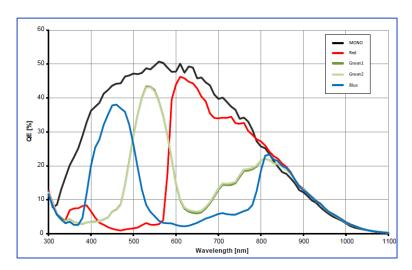
**Figure 66:** Python CMOS typical color spectral response (with micro lens and cover glass)
