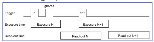
Figure 56: "Fast" Trigger Mode (Internal Exposure Control)
