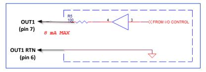
Figure 6: OUT1 LVTTL electrical connection
