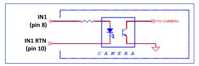
Figure 4: IN1 electrical connection
