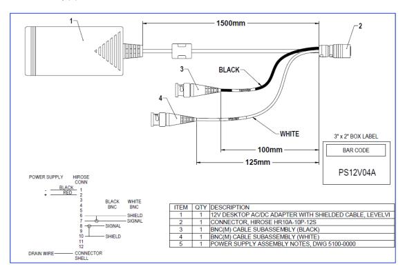
Figure 11: PS12V04A Power Supply assembly
