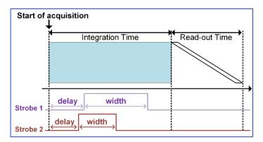
Figure 58: Strobe positioning with respect to exposure start
