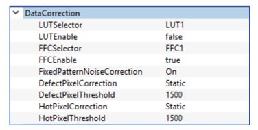
Figure 37: Data correction parameters.
