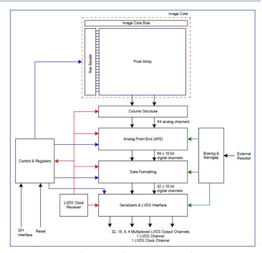
Figure 64: Typical CMOS image sensor architecture
