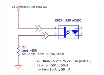
Figure 9: High side load driver
