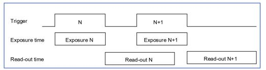
Figure 57: "Fast" Trigger Mode (Pulse Width Exposure Control)
