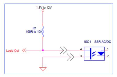
Figure 7: Open drain logic driver
