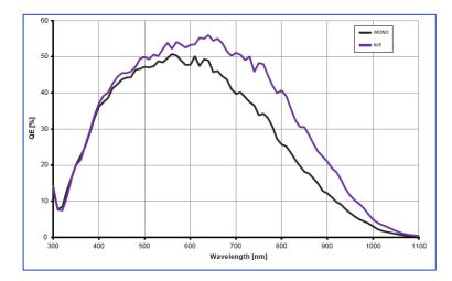
**Figure 65:** Python CMOS mono spectral response (monochrome with the cover glass) for monochrome and enhanced NIR versions
