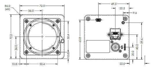
Figure 14: Mechanical drawings of GEV-C5180, GEV-C4181, and GEV-C4180 cameras
