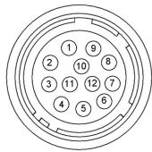
Figure 3: Power and I/O Connector Pin-outs
