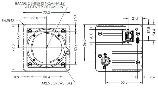
Figure 15: Mechanical drawings of 10G-C5180, 10G-C4181, and 10-C4180 cameras
