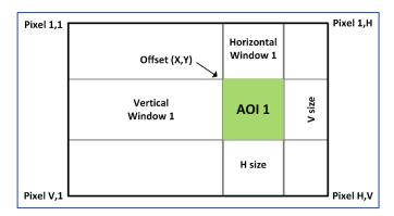
Figure 52: Horizontal and vertical window positioning
