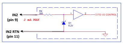
Figure 5: IN2 electrical connection
