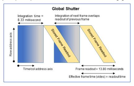
Figure 51: Global Shutter with 8.33 ms exposure time
