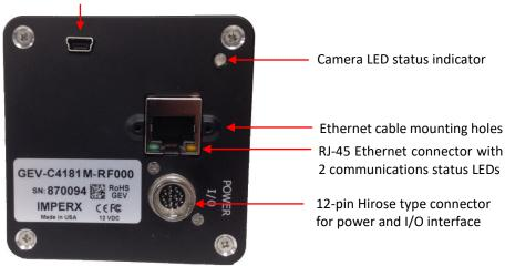
Figure 1: GEV-C5180, GEV-C4181, and GEV-C4180 camera back panel
