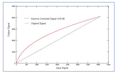
Figure 62: Gamma corrected video signal
