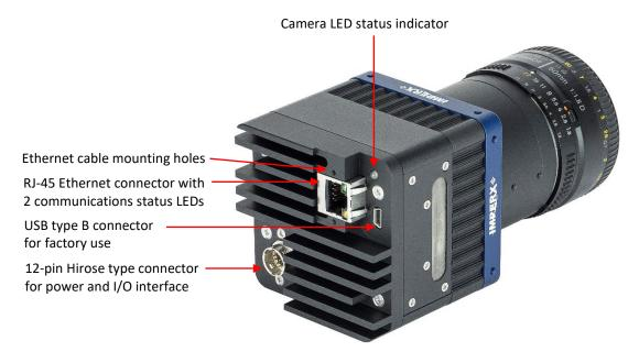
Figure 2: 10G-C5180, 10G-C4181, and 10G-C4180 camera back panel
