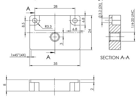
**Figure 40:** P67-C1911, P67-C2010, P67-C2410, P67-C3210, P67-C4010, P67-C4110 cameras mounting plate
