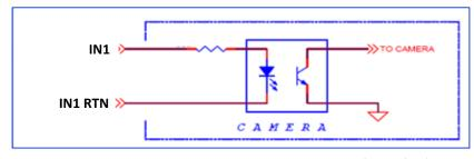
Figure 16: Opto-isolated input electrical schematic (simplified)
