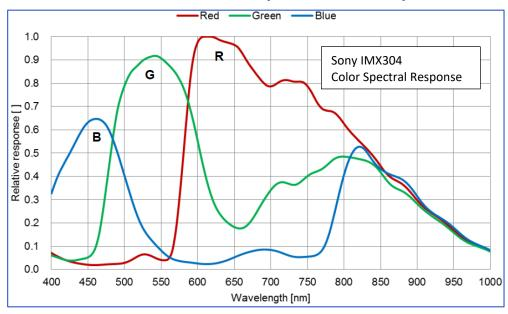
Figure 107: Cheetah C4110 Color Spectral Response
