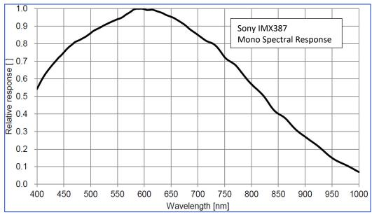
Figure 112: Cheetah C5410 Monochrome Spectral Response
