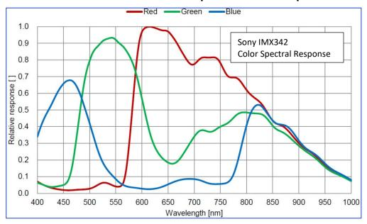
Figure 113: Cheetah C6410 Color Spectral Response
