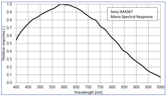
Figure 110: Cheetah C4410 Monochrome Spectral Response
