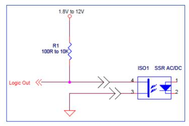
Figure 19: Out2 Open drain logic driver circuit
