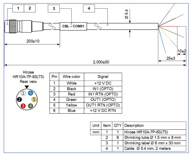
Figure 11: CBL-COM01 cable for use with C2000 and C2400 cameras (ordered separately)
