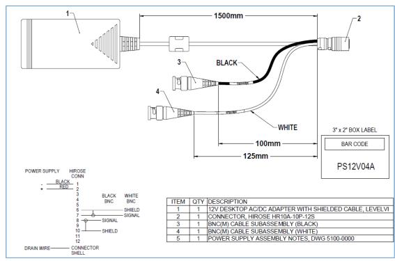
Figure 10: PS12V04A Power Supply assembly
