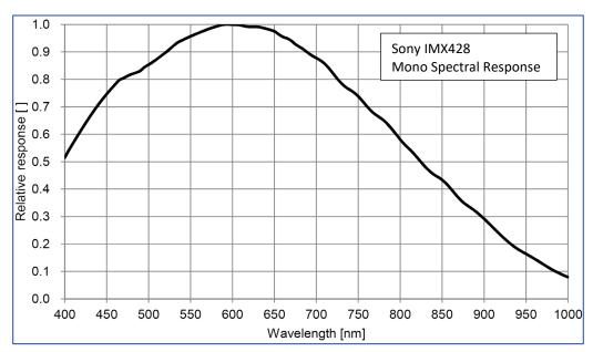
Figure 104: Cheetah C3210 Monochrome Spectral Response
