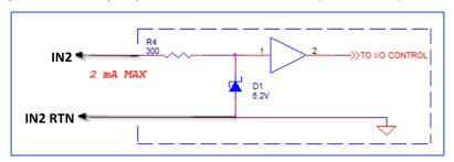
Figure 17: TTL input electrical schematic (simplified)
