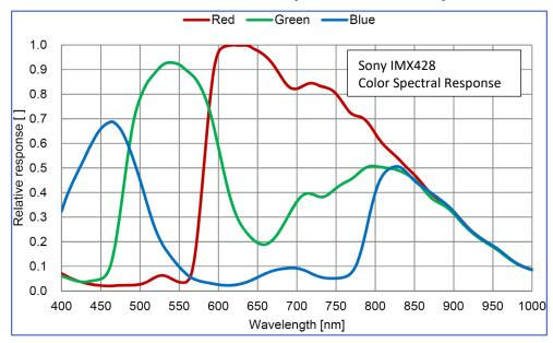
Figure 103: Cheetah C3210 Color Spectral Response
