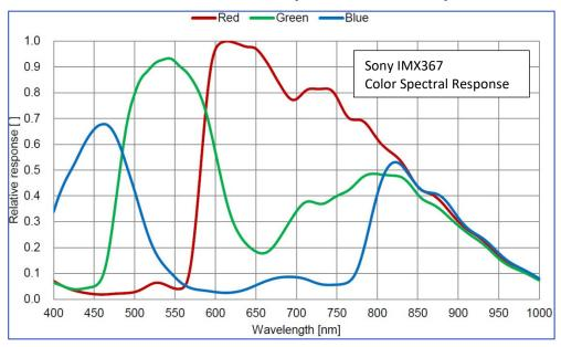
Figure 109: Cheetah C4410 Color Spectral Response
