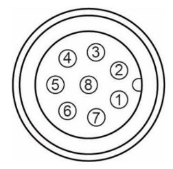
**Figure 7:** BULGIN PXMBNI12RPM08APCM12 connector pin-outs (P67-C1911, P67-C2010, P67-C2410, P67-C3210, P67-C4010, and P67-C4110 cameras)
