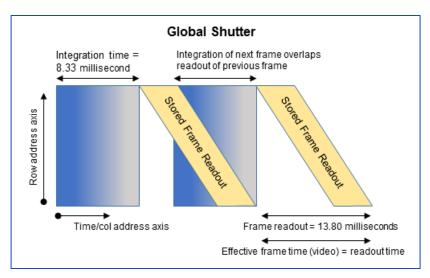
Figure 90: Global Shutter with 8.33mS exposure time
