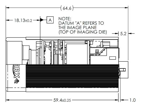
Figure 24: Bottom and Side views of the C2000 and C2400 cameras
