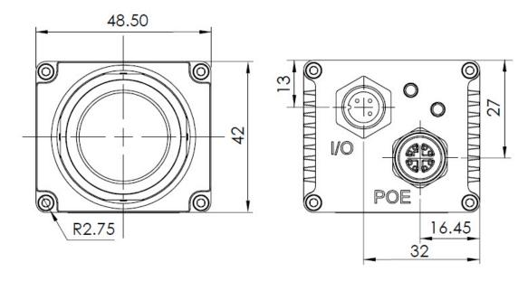
**Figure 35:** Front and Back views of the P67-C1911, P67-C2010, P67-C2410, P67-C3210, P67-C4110 cameras
