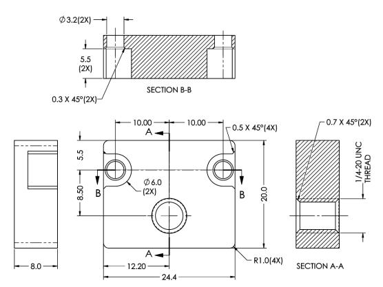
Figure 25: C2000 and C2400 Camera mounting plate
