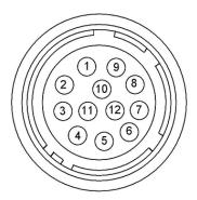
Figure 4: 12-pin Hirose Connector Pin-outs (POE-C1911, POE-C2010, POE-C2410, POE-C3210, POE-C4010, POE-C4110, POE-C4410, POE-C5410, and POE-C6410 cameras)
