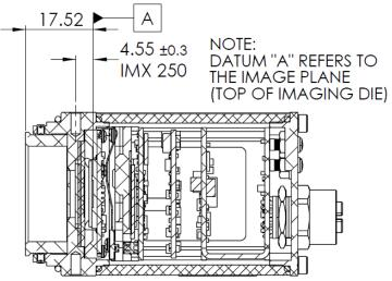
**Figure 36:** Mechanical drawings of the P67-C1911, P67-C2010, P67-C2410, P67-C3210, P67-C4010, P67-C4110 cameras
