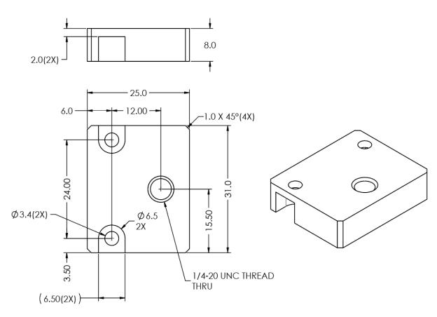
**Figure 29:** POE-C1911, POE-C2010, POE-C2410, POE-C2410Y/Z, POE-C3210, POE-C4010, POE-C4110, and POE-C4110Y/Z cameras mounting plate
