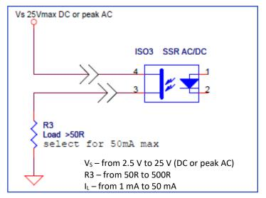
Figure 21: Out2 High side load driver circuit
