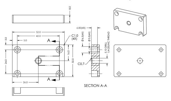
Figure 33: C4410, C5410, and C6410 Cameras Mounting Plate
