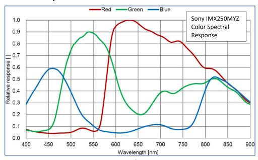
Figure 101: Cheetah C2410Y/Z Color Spectral Response
