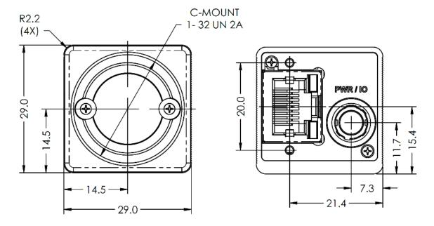
Figure 23: Front and Back Views of the C2000 and C2400 cameras
