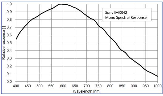
Figure 114: Cheetah C6410 Monochrome Spectral Response
