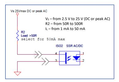
Figure 20: Out 2 Low side load driver circuit
