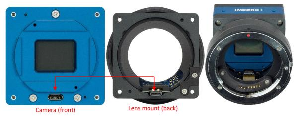
Figure 15: The camera (left) and Canon EF lens mount (center) connect internally
