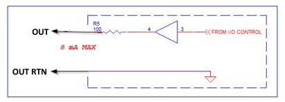
Figure 18: TTL output electrical schematic (simplified)
