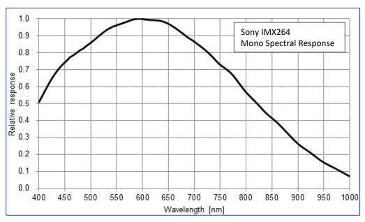
Figure 100: Cheetah C2400 and C2410 Monochrome Spectral Response
