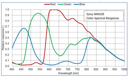
Figure 95: Cheetah C1911 Color Spectral Response
