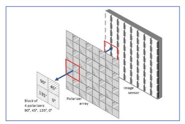
**Figure 94:** The POE-C2410Y/Z and POE-C4110Y/Z cameras micro-polarizer blocks image obscuring light waves from reaching the sensor
