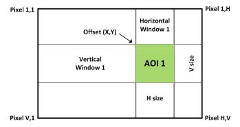
Figure 93: Horizontal and vertical window positioning
