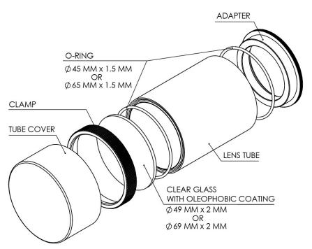
Figure 39: IP67 C-Mount Lens Tube, exploded drawing
