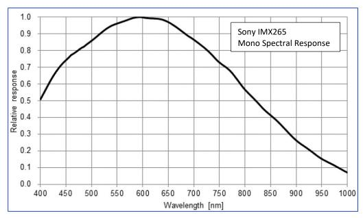
Figure 98: Cheetah C2000 and C2010 Monochrome Spectral Response
