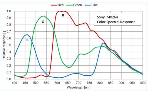
Figure 99: Cheetah C2400 and C2410 Color Spectral Response
