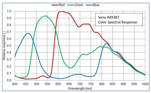
Figure 111: Cheetah C5410 Color Spectral Response
