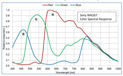
Figure 105: Cheetah C4010 Color Spectral Response
