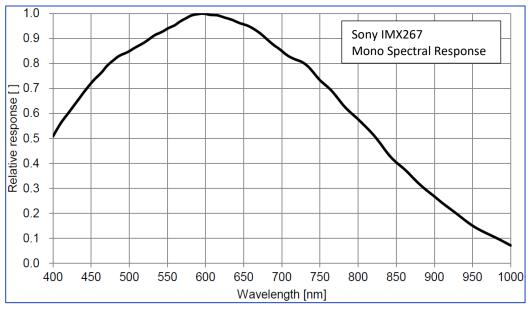
Figure 106: Cheetah C4010 Monochrome Spectral Response
