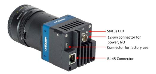
Figure 5: POE-C4410, POE-C5410, and POE-C6410 camera back panel connectors
