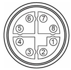
**Figure 8:** MACOM MMT361A315 connector pin-outs (P67-C1911, P67-C2010, P67-C2410, P67-C3210, P67-C4010, and P67-C4110 cameras)
