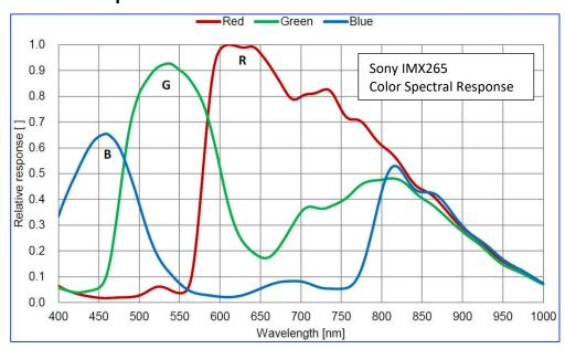
Figure 97: Cheetah C2000 and C2010 Color Spectral Response
