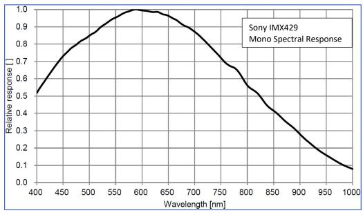
Figure 96: Cheetah C1911 Monochrome Spectral Response
