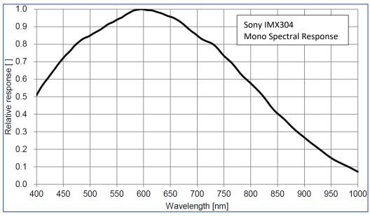
Figure 108: Cheetah C4110 Monochrome Spectral Response
